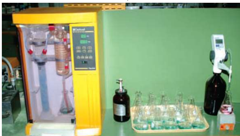
រូបភាព ៣.៧. Automatic distillation unit (Kjeldahl) and automatic burette for titration
