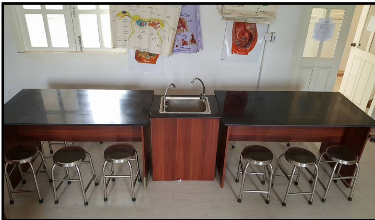
Figure 3.13 – Island Workstation: The proposed Island Workstation in a science lab sits two groups of 6 students on either side of a sink with two faucets that can be used in common. The sink stand also includes a cabinet at its back that can be used for storage. This work station is designed for use with short stools made of chrome or wood. Work stations are made of heavy pressed wood frames and with Mahogany color formica veneer. Work station tops are made of black marble with high gloss to resist any chemical spills. Sinks may be made of high-quality stainless steel or ceramic. Stools are made of high gloss chrome with hard rubber leg caps to prevent rubber marks on the floor.
